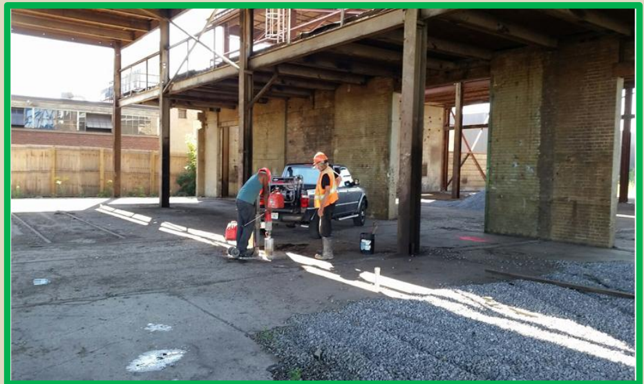
Environmental soil sampling. Old fuel storage facility
