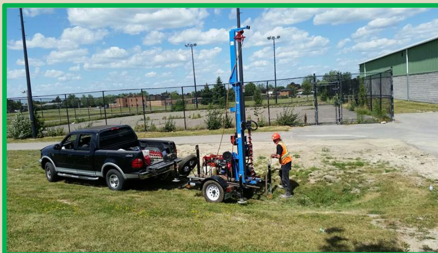
Soil testing for contaminant remediation
